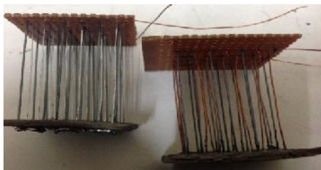
TEGs made using commercially available materials
