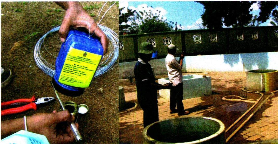
Left: Installing passive radon detectors in a custom built housing which provides protection from the elements. Right: Investigating the thermal springs at Maha Oya
