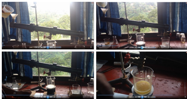
Figure 3: Physical reactor option 1, oil can be collected from the second compartments and water can be collected from the third compartment and membrane is fixed in the union between 2 and 3
