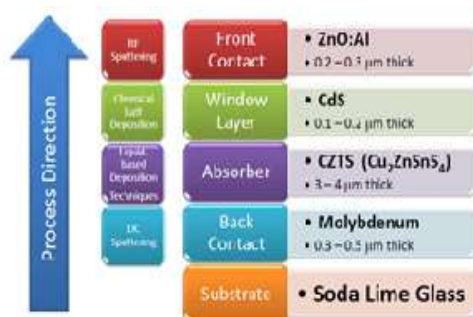
Figure 2: CZTS Solar Cell Device Structure and Process Direction
